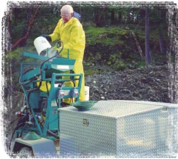
On-site processing of ore samples with the Knelson Prospecting Trailer (includes KC-MD7.5 with a vibrating screen, generator and equipment for field testing).
