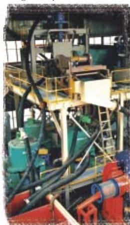
Turnkey gravity concentration module, supplied and installed by Knelson Gravity Solutions. (KGS)
