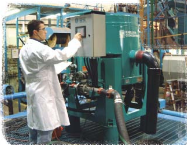
KC-XD20 machine complete with Knelson ICS 2.0 automation.
