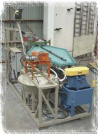
Knelson's Automated Tabling System (ATS) is a chemical-free, fully automated, multiple-pass tabling system used to maximize table gold recovery.
